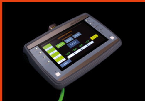
Portable control panel displaying real-time pressure data.
